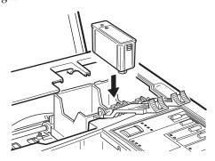
Be sure to install both ink cartridges. The printer will not work if only one cartridge is installed.
